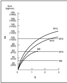
1. Fastening time (second) 2. Fastening torque
