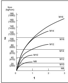
1. Fastening time (second) 2. Fastening torque
