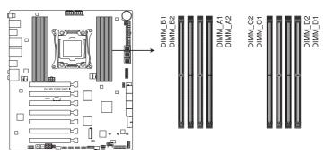
Pro WS X299 SAGE II 288-pin DDR4 DIMM socket
