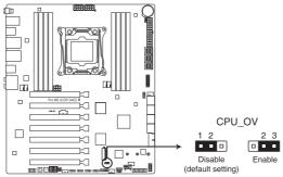
Pro WS X299 SAGE II CPU Over Voltage jumper
