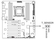
Pro WS X299 SAGE II Thermal Sensor connector
