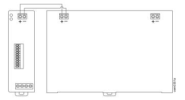
Connect the battery wires to the battery terminals (refer "Front Panel Features" for details).
