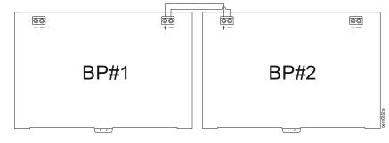
Connect the battery wires to the battery terminals (refer "Front Panel Features" for details).
