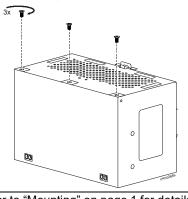
a. Mount the battery pack on the DIN rail. Refer to "Mounting" on page 1 for details. b. Connect all the wires to the battery pack (disconnected in step 1)
