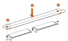
Tighten the screws with a screwdriver to secure the M.2 heatsink into place. Please do not overtighten the screw as this might damage the module and M.2 heatsink.
