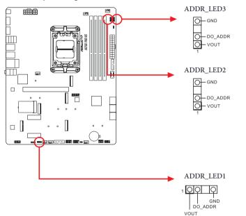
Connect your Addressable RGB LED strips to the Addressable LED Headers (ADDR\_ LED1 / ADDR\_LED2 / ADDR\_LED3) on the motherboard.
