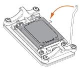
Make sure the CPU is aligned with the  $\square$ socket before locking it into place.
