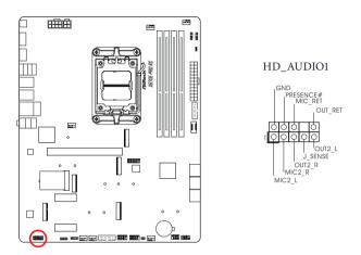
High Definition Audio supports Jack Sensing, but the panel wire on the chassis must support HDA to function correctly. Please follow the instructions in our manual and chassis manual to install your system. Chassis/Water Pump Fan Connectors
