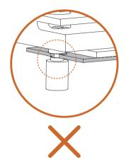
Incorrect Installation: The SSD's PCB sits between M.2 heatsink and standoff. Do not continue.
