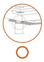
Correct Installation: The SSD's PCB is in proper place, and the M.2 heatsink can be screwed in.
