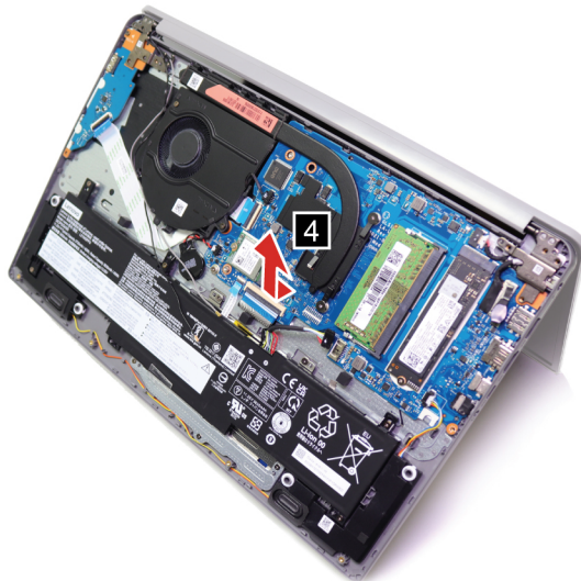
Figure 35. Remove the upper case
