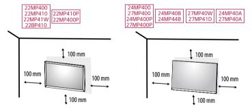
To install the monitor to a wall, attach a wall mounting bracket (optional) to the back of the monitor. Make sure that the wall mounting bracket is securely fixed to the monitor and to the wall.
