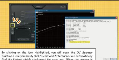
find the highest stable clockspeed for your card. When the process is done, click Apply and your GPU is now running at a higher speed.
