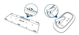
Connect the wireless dongle for keyboard and mouse to a USB port to automatically pair both devices to your ASUS All-in-One PC
