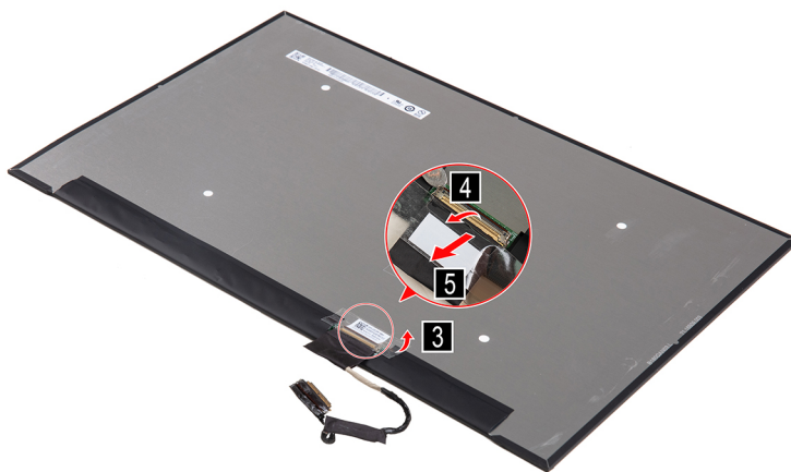
Figure 33. Disconnect the EDP cable
