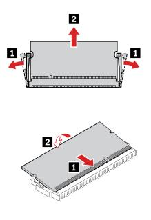
**Note:** During the installation, ensure that you align the memory module to the slot and press down on both ends until the latches are fully engaged with a click.
