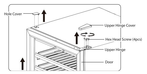
**2.** Remove the Hole Cover and Upper Hinge Cover on top side using a flat-head screwdriver. Remove the
