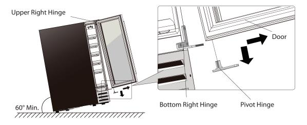
**3.** Unscrew the Upper Right Hinge and Bottom Right Hinge from the cabinet. Keep them well for door reinstallation.
