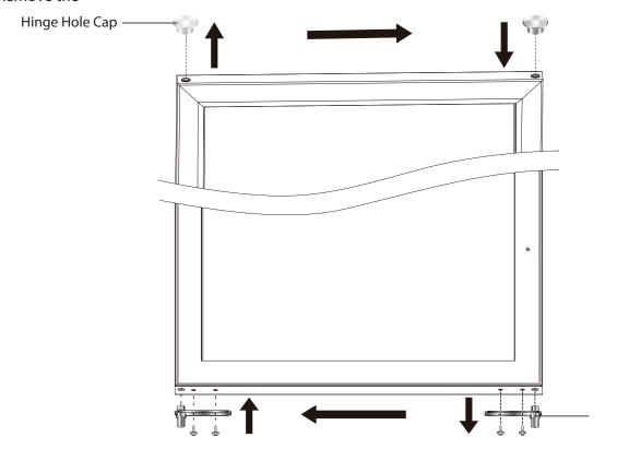
**3.** Remove the Bottom Hinge Cover by prying it off gently with small flat screwdriver. Remove the Bottom Hinge by unscrewing the Hex Head Screw (4pcs). Unscrew the Pan Head Screw (4pcs) from bottom left side. Now move the Bottom Hinge to the bottom left side and screw it tightly with the Hex Head Screws (4pcs). Move the Pan Head Screw (4pcs) to the bottom right side and screw it.
