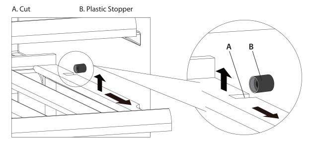
• For a model with Telescopic Rail, pls. lift the whole Shelf upwards horizontally to get it off from the 4 Locating Pins of Telescopic Rail.
