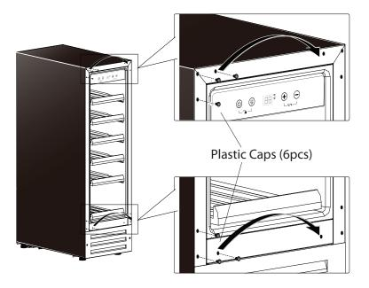
**5.** Install the Upper Left Hinge and Bottom Left Hinge to the left side of the cabinet. Make sure the screws are tightened.
