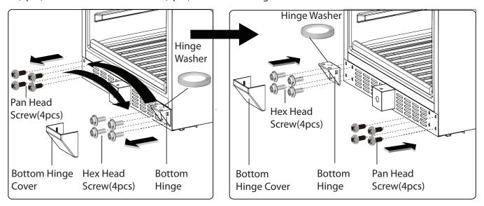
**4.** Hold the Door carefully with your assistant and place it on the top of Bottom Hinge, make sure the Pivot Hinge is at correct place through the Hinge Washer. Insert the pin of the Upper Hinge into the Bushing on the top right and fix it with Hex Head Screw (4pcs). Cover the Upper Hinge and Bottom Hinge with Upper Hinge Cover and Bottom Hinge Cover. Cover hinge screw holes on the top right with the Hole Cover.
