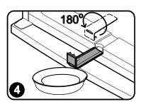
FREEZER COMPARTMENT should be thawed not less than twice a year or when a layer of ice thicker than 5 mm forms in it. Do the actions below in the order they are listed:
