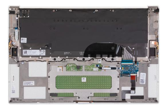
Place the palm-rest and keyboard assembly on a flat surface.
