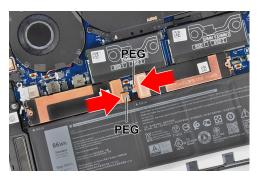
3. Slide and remove the solid-state drive 1 from the solid-state drive slot.
