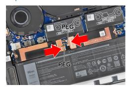
Replace the screw (M2x2) that secures the solid-state drive thermal bracket and the solid-state drive 2 to the system board.
