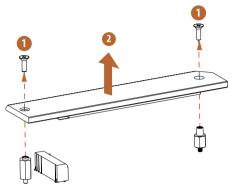
Before installing a M.2 SSD module, please loosen the screws to remove the M.2 heatsink.
