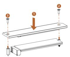
Tighten the screws with a screwdriver to secure the module (if your M.2 SSD module is Type 2280) and M.2 heatsink into place in the order shown. Tighten screw opposite the M.2 connector first (2), and then tighten the one next to the M.2 connector (3).
