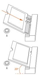
Gently insert the WiFi/BT PCIe WiFi module or Intel\* CNVi (Integrated WiFi/BT) into the M.2 slot. Please be aware that the module only fits in one orientation.
