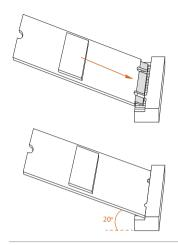
Align and gently insert the M.2 SSD module into the M.2 slot. Please be aware that the M.2 SSD module only fits in one orientation.
