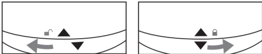
Turn the battery compartment lid. Insert 2 AAA batteries in accordance with the marking. Reapply the battery compartment lid, ensuring correct alignment.
