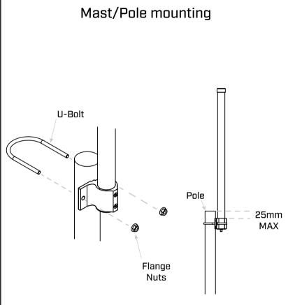
Place the antenna against the tip of the pole. Attach the U-Bolt to the pole and place it through the mounting holes of the antenna. Use the included Flange Nuts to secure the antenna in position. Compatible with pole sizes from 25-50mm. Best performance will be achieved if antenna is mounted less than 25mm from the top of the pole.
