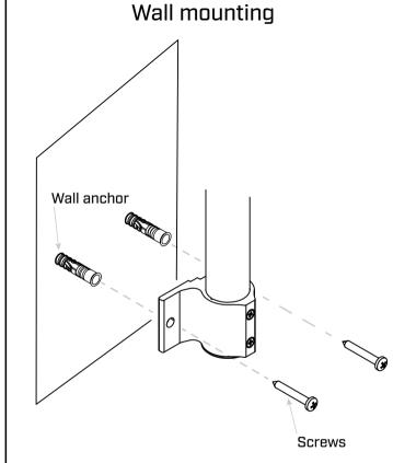
Place the antenna against the wall, mark the mounting holes.
