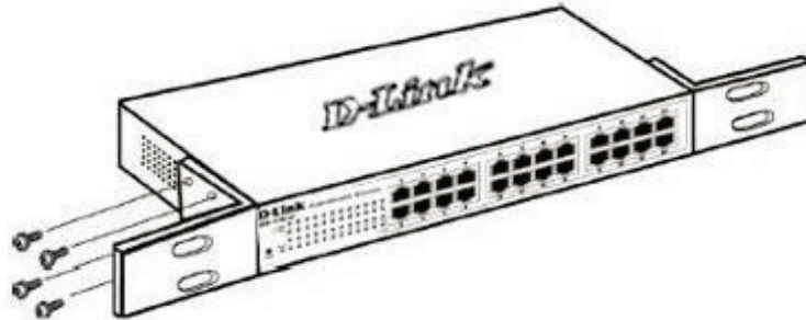
Figure 3-2 – Attach the mounting brackets to the Switch
