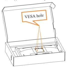
Step 5: Attach the LCD display to the wall, and follow the instructions in the wall-mounting kit. For use only with UL Listed Wall Mount Bracket with minimum weight/load: 8kg
