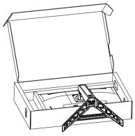
Step 3: Remove the base and stand from the monitor, refer to "Detaching the monitor base and stand" on page 2-11.
