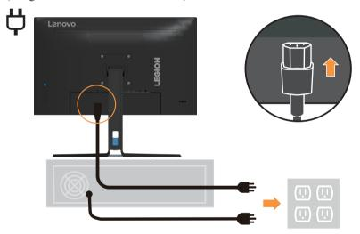
7. Connect the cables with cable clip.
