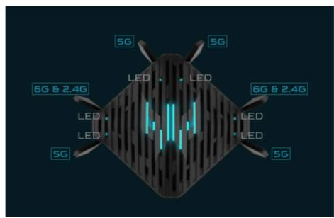
Note 1: Please make sure that your mobile device or computer is wirelessly connected to the router. The feature is not applicable when connected via Ethernet LAN. Note 2: Four signal strength LEDs will be ON when the client is associated with 5GHz and calibrated. If the client is associated with 2.4GHz or 6GHz, only two signal-strength LEDs will be ON.
