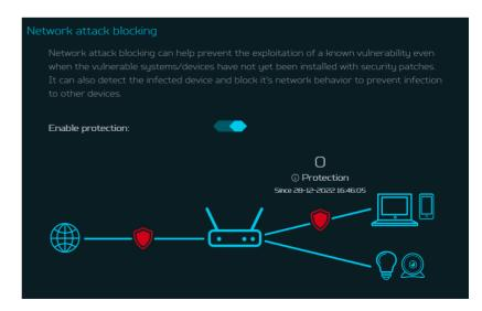
Enabling IoT security protection feature detects and blocks harmful connections from compromised IoT devices by using Trend Micro's smart protection network.
