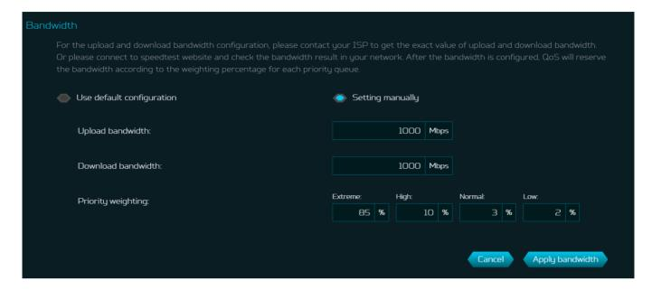
You may select "use default configuration" and click on "Apply bandwidth". you can select "setting Otherwise, manually" and enter the required upload and download bandwidth with priority weighting.
