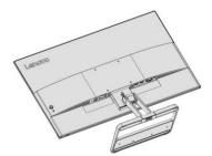
Step 3: Remove the base and stand from the display, see "Removing the Display Base and Support Arm" on pages 2-9.
