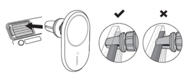
**NOTE:** Do NOT clip the device on the car vent when your heater is ON.
