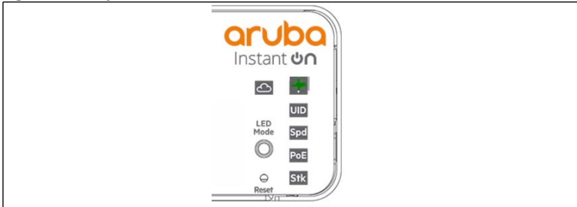
Figure 7. System LED Indicators
