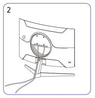
Put both cables in the cable holder on the stand (HOLDER-STAND CABLE) to organise the cables, as shown in the figure. Assembly is complete.
