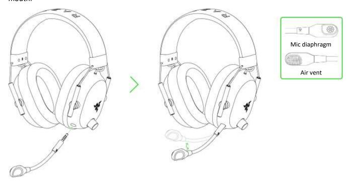
The recommended mic-to-mouth distance for optimal sound capture is 1.5 cm to 3 cm (0.59 in to 1.18 in).
