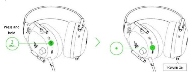
3. Wait until the status indicator briefly becomes static green, indicating that the headset is connected to the wireless USB dongle
