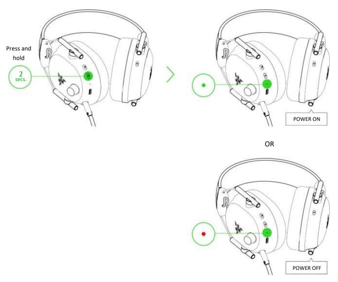
1 The headset will power on using the last active audio source before power off.
