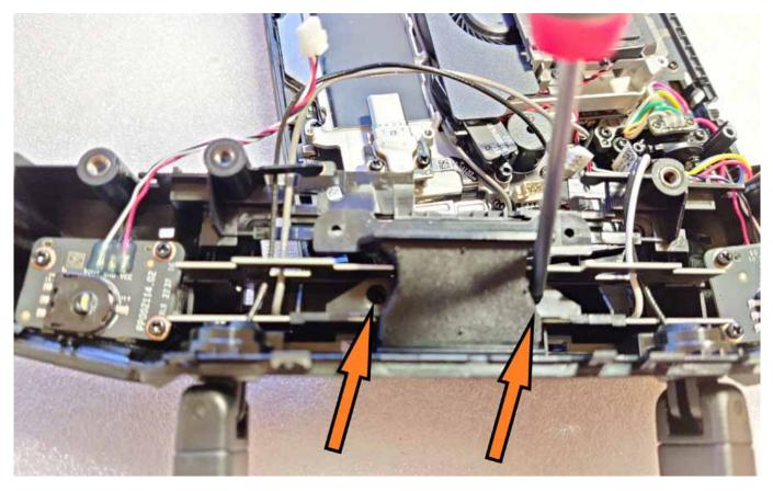
...and remove the middle plastic part, that is holding the antenna boards.
