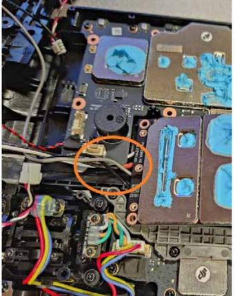
The antenna cables are located under the transmission module, secured with a metal bracket. Make a picture to remember the order of cables plugged in 4 ports.
