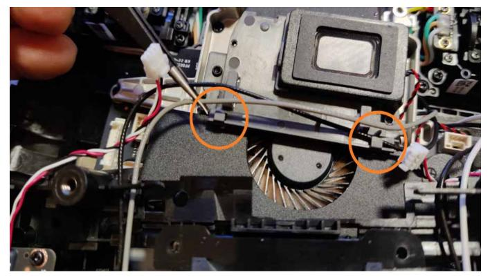
Remove 2 screws from the antenna module in detached top panel...
