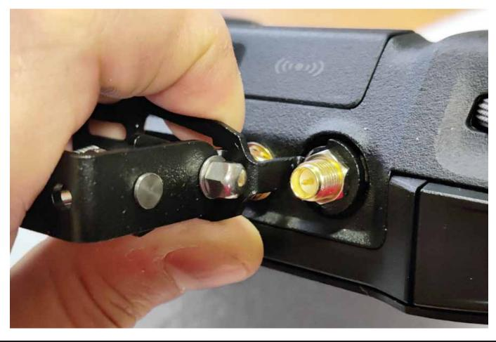
Using the attached 15cm RP-SMA -> RP-SMA cables, connect two outer ports on the controller with 2 outer ports at the antenna (marked as P1 and P2). Then connect two inner ports with two inner ports at the antenna.
