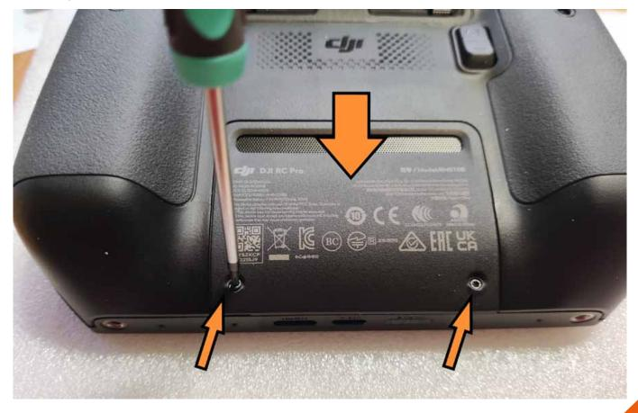
Re-install 2 screws located at the bottom holes.
