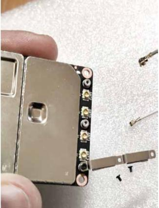
It's time to remove the internal antennas and their screens. In order to remove these, first you'll have to remove the PCB under the control wheels on the top-left and top-right panel. Put the removed PCB's in a safe place.
