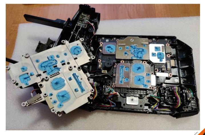
Remove 2 U.FL plugs from their sockets, and put the fan part aside in a safe place.
