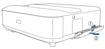
Pull the air filter out of the projector.
