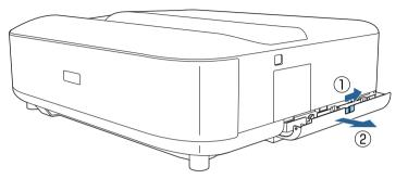
Pull the air filter out of the air filter cover.
