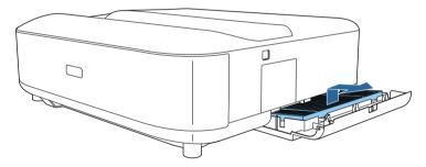
Vacuum the front of the air filter (the side with the tabs) to remove any remaining dust.
