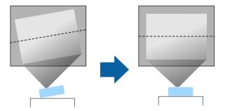
• If the image is tilted, rotate the front feet to adjust their height.
