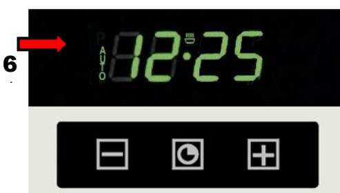
In our example, the oven should switch on at **12:25 (6)** with the functions “Grill + Hot air circulation” and switch off at **12:55** according to your setting.
