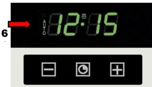
The end of the countdown is indicated by a double acoustic signal at intervals of 2 seconds. The flashing symbols inform you that the oven is switched off completely.
