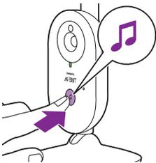
To activate the lullaby feature from the baby unit, press the lullaby on/off button on the baby unit.
