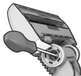
3. Unscrew the wheel axis and clean all parts. Refit in reverse order.
