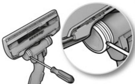
2. If the wheels are stuck, clean them by removing the wheel cap with a small screwdriver.
