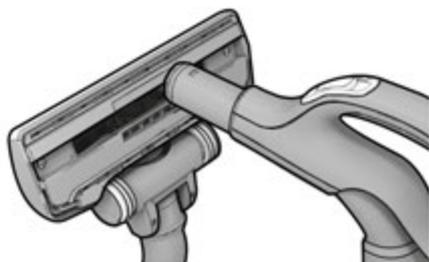
1. Disconnect the nozzle from the tube. Use the hose handle to clean the nozzle.
