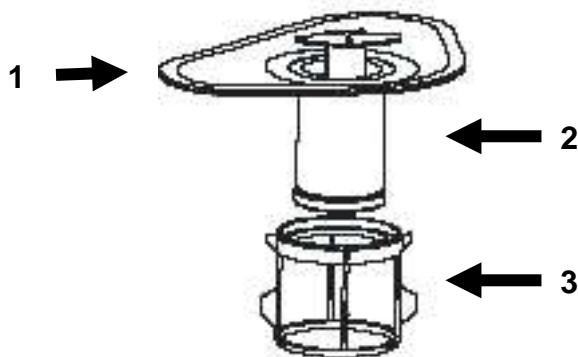
For your convenience, we have placed the drain pump and filtering system within easy reach inside the tub. The filter prevent larger remnants of food or other objects from getting inside the pump. This residue can occasionally clog up the filters.
