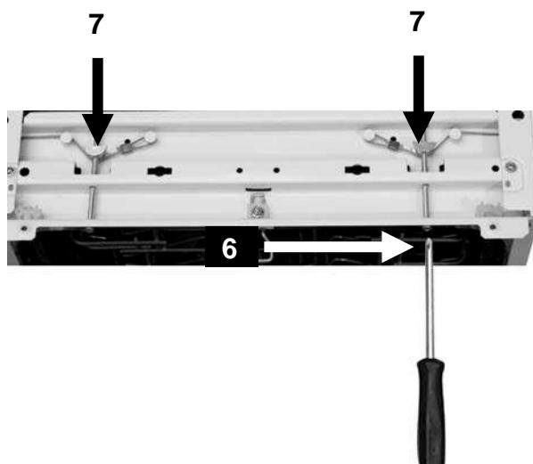
The door springs are set at the factory to the proper tension for the outer door. If aesthetic wooden panel are installed, you will have to adjust the door spring tension. Rotate the adjusting screw 6 to drive the adjustor 7 to strain or relax the steel cable.
